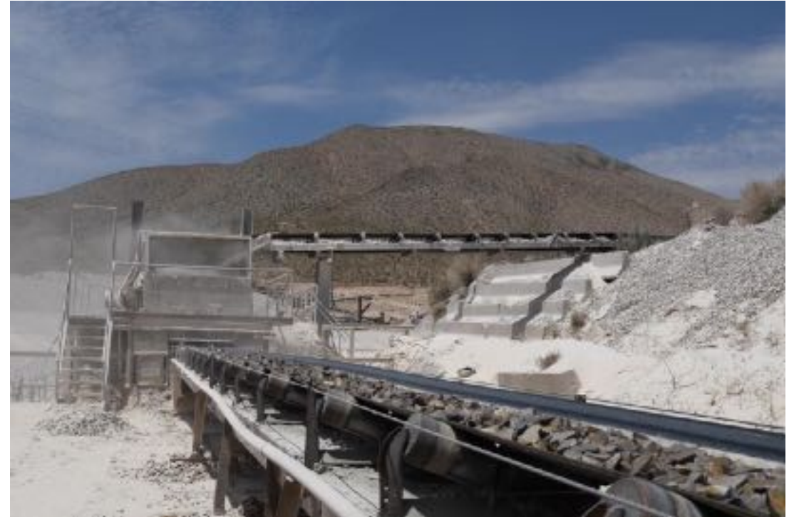
Figure 1.10a - Crushed rock is deposited at washer. Figure 1.10b - Washed rock is transported by conveyor to end of conveyor line where it is deposited in piles and allowed to dry. Photos by BK Darling.
