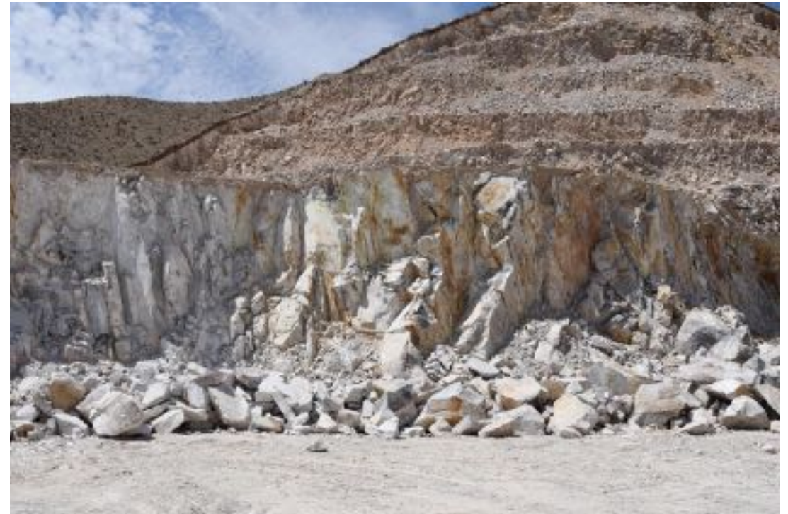
Figure 1.05a – Sample of quartz rhyolite porphyry from main quarry.. Figure 1.05b - View of debris at base of quarry wall. Note benches cut above quarry wall.
