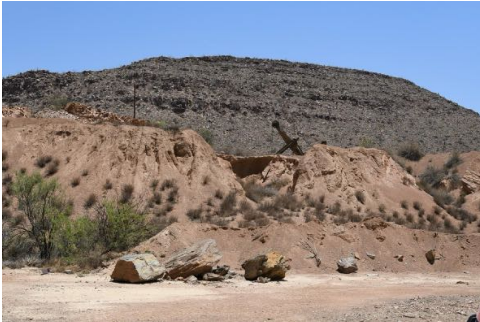
Figure 2.06 – Old area of main pit at Desert Rock quarry. The hill in background is composed of Campgrande and Cox formations (Cretaceous). The pit and the hill are separated by the Hillside fault (see Figure 2.01 ). Photo by BK Darling.
