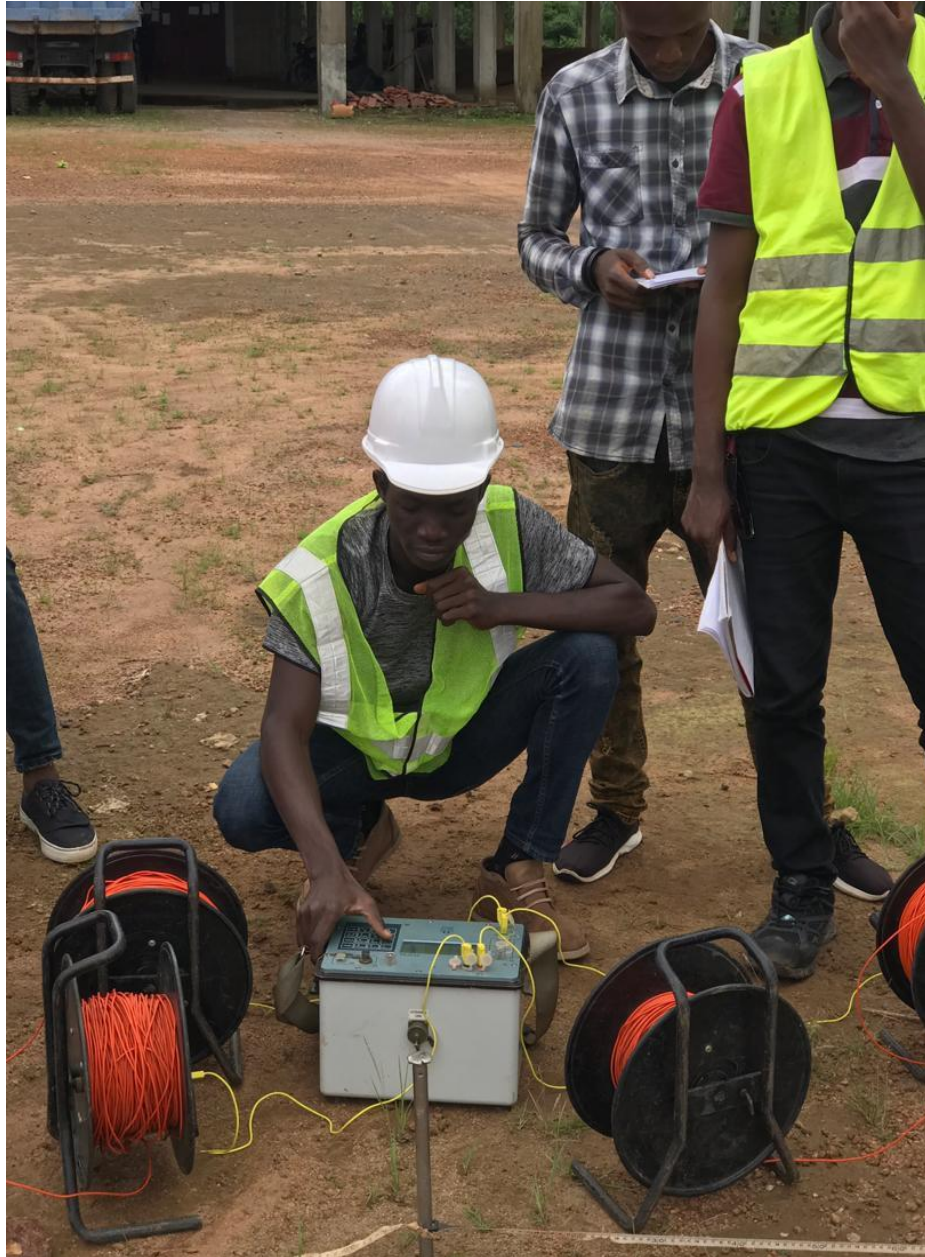
Figure 3. 11 Image of author operating the Syscal Junior Resistivity machine
