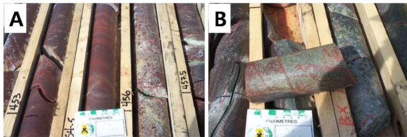
Fig. 3. Core samples of uranium ores consisting mainly of hematite and chlorite developed along the unconformity plane.
