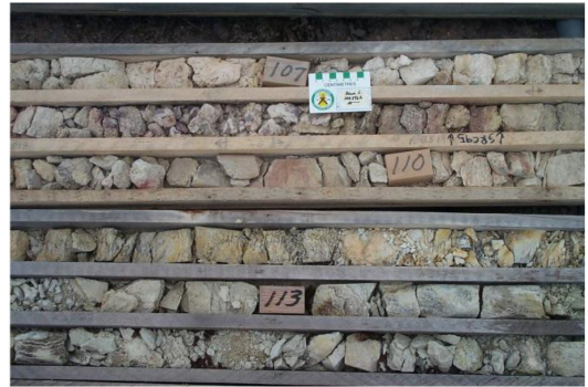
Fig. 6. Core samples from alteration zone consisting of various altered minerals such as chlorite, illite, and dickite.
