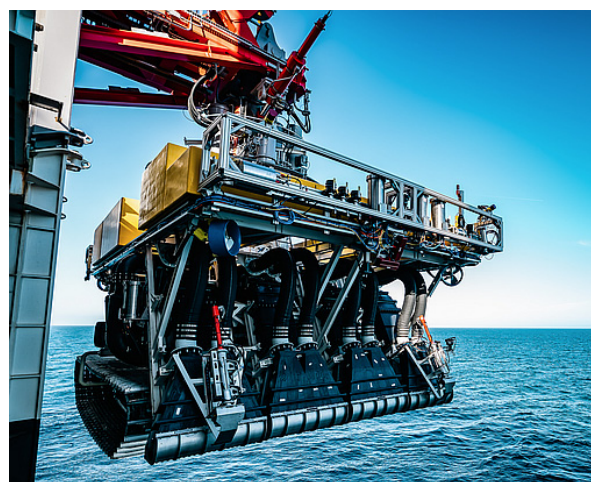
Figure 4. Underwater deployment of the Allseas-designed pilot nodule collector [38].
